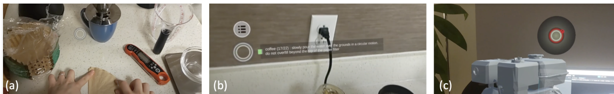
Figure 1: Our non-humanoid ECA in two testbed environments: (a–b) recipe guidance and (c) equipment maintenance. (a) In an ‘idle’ state, the agent consists of two concentric rings. (b) When the user looks at the agent, it displays task or notification details. (c) To notify the user about new information, such as a warning, a halo [3] attracts the user’s attention until they look at the agent.
